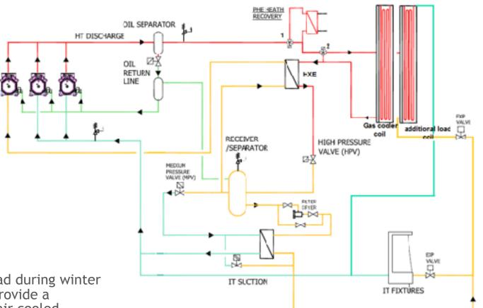
For stores where cooling load during winter and night could be low to provide a sufficient heating load, an air cooled evaporator, integrated in the gas cooler coil, is connected at the unit suction side as additional load.
