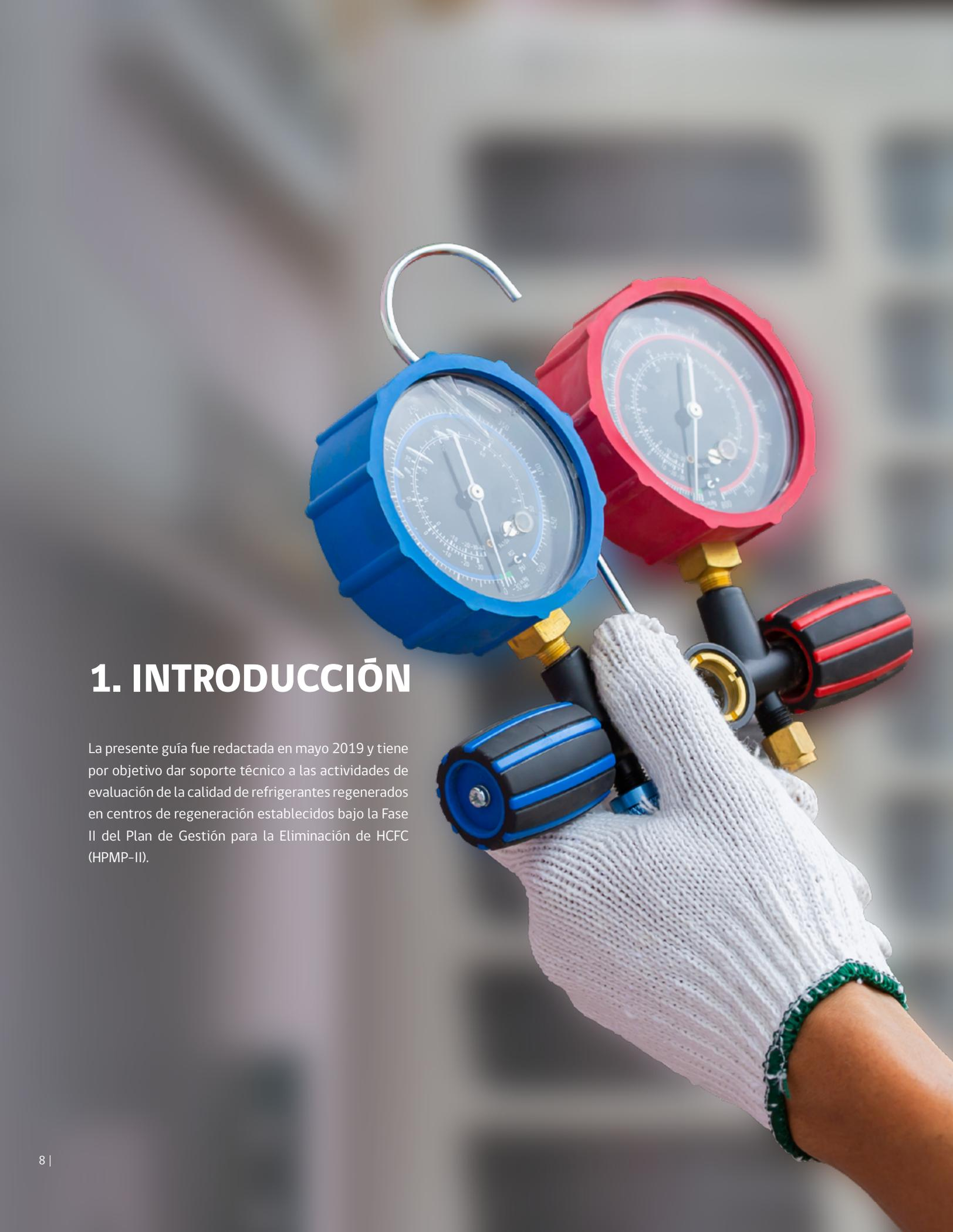
A hand wearing a white knitted glove holds a manifold gauge set. The gauge set consists of two circular gauges, one blue and one red, with multiple ports and valves. The background is a blurred outdoor scene with trees and a building.
